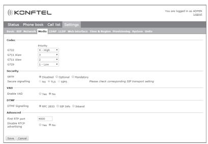
The media settings determine how audio is sent between the devices. The devices negotiate via SIP before a call is connected. All devices must support the same media types, codecs and security settings.
