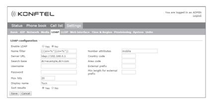
Konftel 300IPx has support for an external phone book, which means it can communicate with a directory server using LDAP (*Lightweight Directory Access Protocol*). The built in search function dynamically filters the content from the LDAP database, based on the search characters the user enter.
