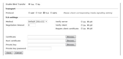
Method The TLS includes a variety of security measures. The methods are defined in the versions of the standard (SSL, SSL v2, SSL v3, TLS v1, TLS v2). The default method is SSLv23, which accepts both SSL v2
