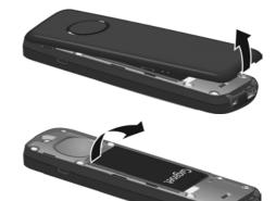
To **change the battery**, insert your fingernail into the notch in the casing and pull the battery upwards.
