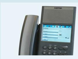
The Dialog 5446 IP Premium features a large, color display with touch screen icons and self-labeling keys. Input is made with a stylus; text commands are not used. The similarity to smartphones is a major factor in increased user-friendliness.
