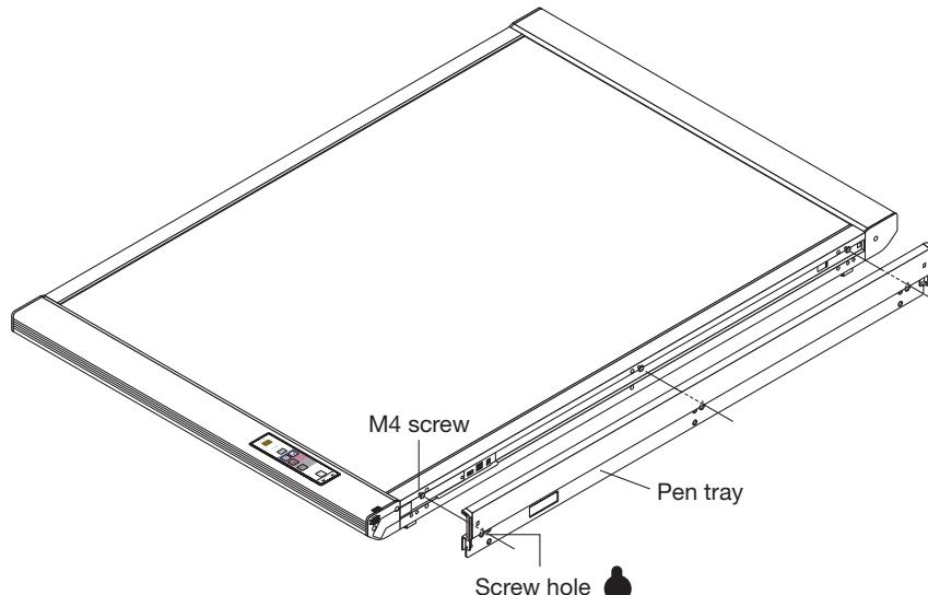
The method of installation differs according to the installation type.
