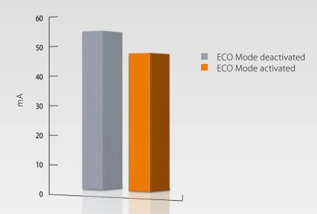
4. For many years, Gigaset DECT handsets have enabled the automatic adjustment of transmission power – depending on the distance to the base station. For example, transmission power is reduced by approximately 60 % at a distance of up to five metres.
